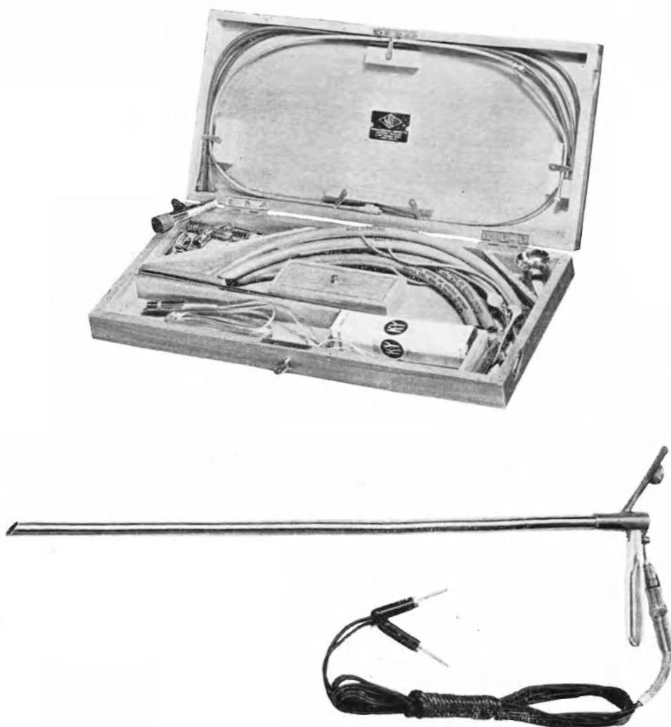
Fig. 816. Bronchoscope outfit, latest pattern suggested by Dr. I. W. Magill, comprising cylindrical stainless steel bronchoscope with connecting leads, three inflatable cuffed tubes, four suction unions, slotted airway, lubricant, three suction catheters, one bronchial occluder with three spare cuffs, all complete with spare bronchoscope bulb in Mahogany case.
